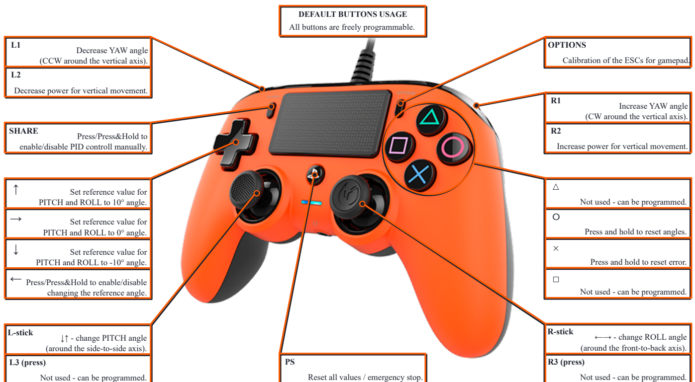
Figure 3: Notation and default functionality description of PS4 gamepad buttons.
